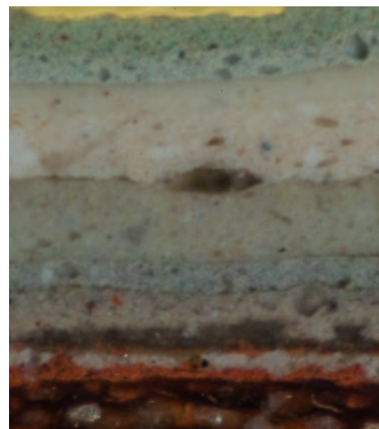
Paint sample cross section from the casing to left of the fireplace in room 203. This sample lacks the tan layer that was present over the red on other samples.
