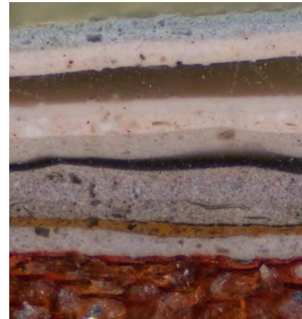
Paint sample cross section from the casing to door #17 in room 205. The initial red is very thin and seems soaked into the wood pores suggesting it was a primer or stain. Than above the first light gray does not have zinc oxide in t.
