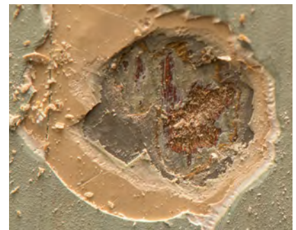
Paint sample in room 205 that has been scraped with a scaple to reveal the surface appearance of the layers. There is only very minimal visible red. As this was not taken with polarized light, the colors are reasonably accurate.
