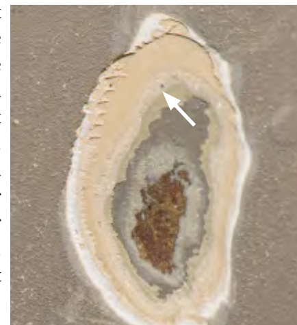
Paint from east post casing in Entry 105. The paint layers on the 1st floor stair woodwork started with the 1927 tan marked with the arrow. The woodwork was repainted several times with similar tans before the 1970s restoration (white primer).
