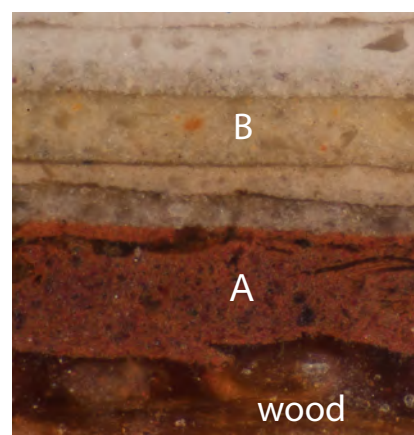
Paint sample cross section from the NE corner post of room 106. "A" marks several layers of the original red oxide paint. "B" marks a later yellowish tan layer that contains zinc oxide dating it to after ca. 1845.
