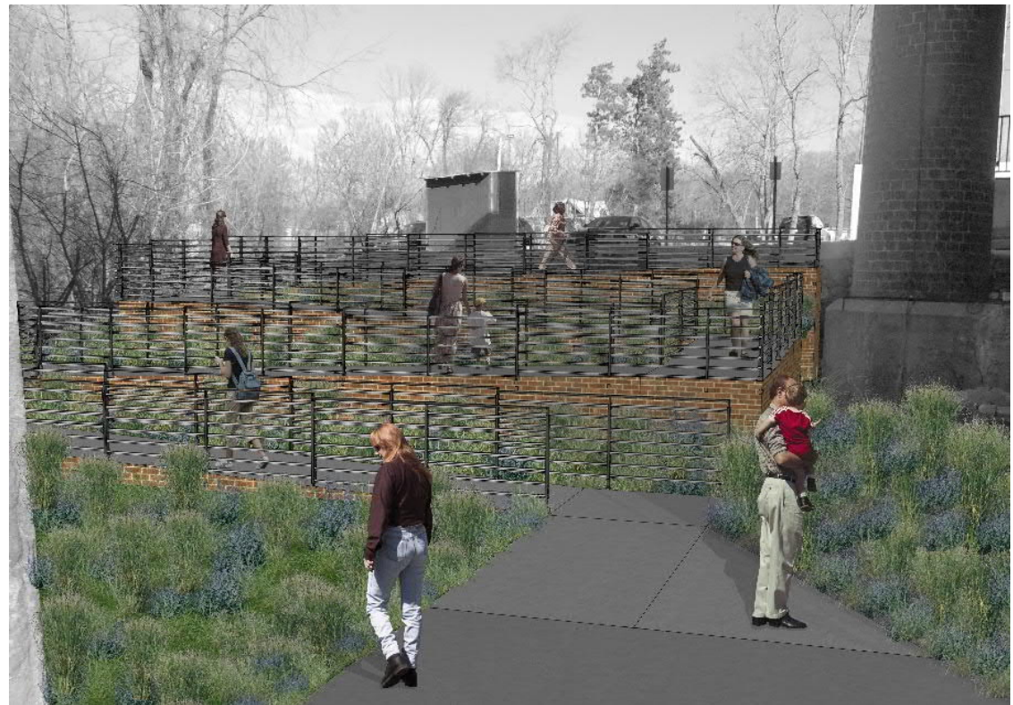
Image 2: Sample rendering of an ADA accessible ramp with integrated bioretention. Image Source: Fuss & O'Neill
